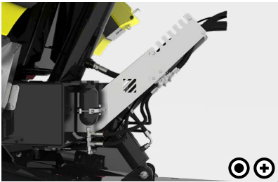
6 Hose duct To ensure a perfect connection to the tractor, all connecting lines are protected in a hose duct.
