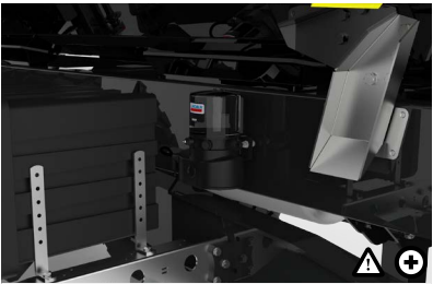
F Central lubrication unit The central lubrication unit provides the entire vehicle with the required lubrication.
