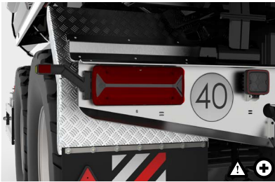
7 All LED lamps All light is produced by LEDs in vehicle lamps that are mounted in protected places and support multi-volt operation (12/24V).
