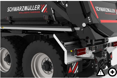
G Lighting package 2 reversing lamps and 4 lateral working lamps for good all-round visibility.
