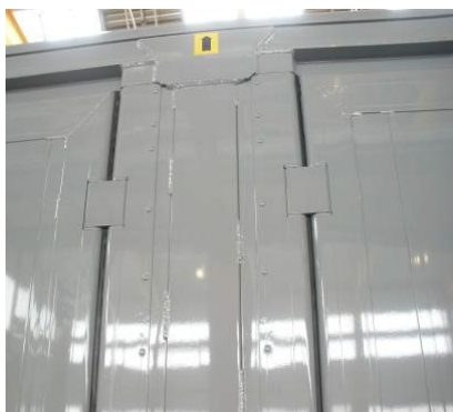
Central posts: Check that the rivets are tight, Check the hinges for operability and damage, Check the hinge mount for damage and that it is tight
