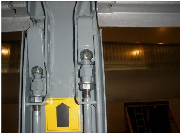
Check latching of pendulum bolt for play and operability
