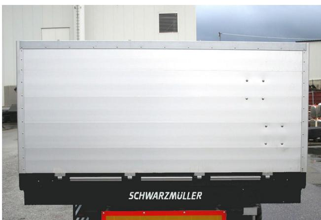
Rear wall: Check that the rivets are tight
