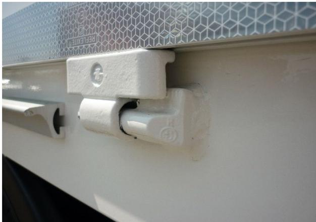
Check the hinges for operability and damage.
