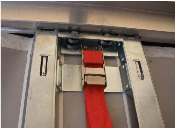
Check top and bottom carriages for wear and correct operability. Check that all rivets and screws are tight
