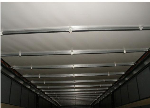
NeLaDa roof tarpaulin: Check for damage and correct attachment
