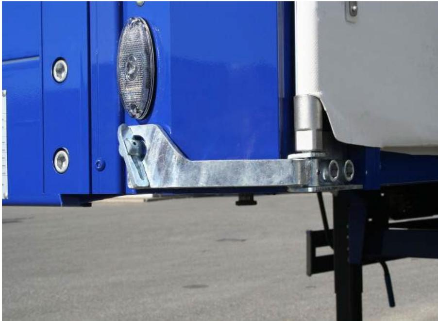
Front quick lock: Check attachment and correct operability.
