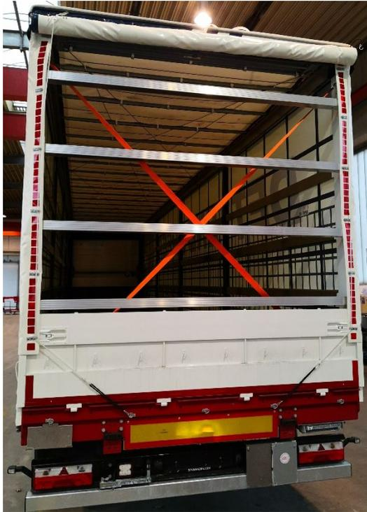
Rejection beam: Check for deflection and holders damage; Replace rejection beam if an obvious deformation is found.
