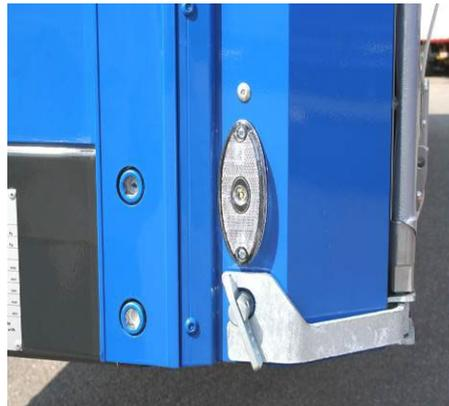
Corner post: Check that all rivets and screws are tight
