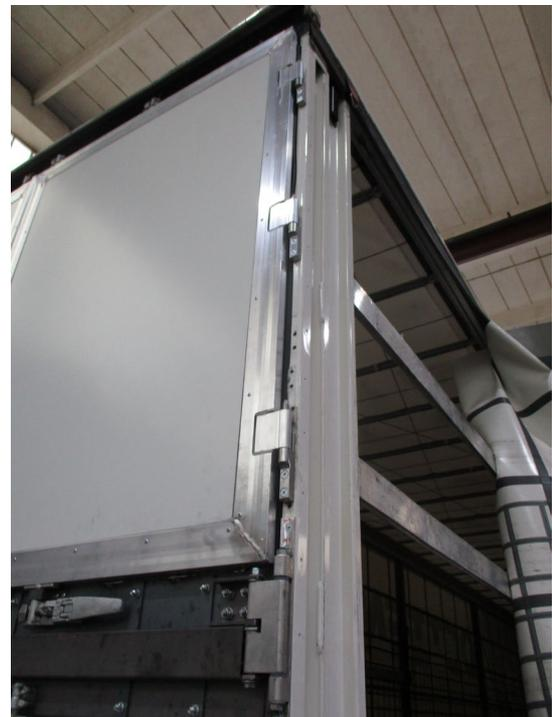
Bottom, central and top rear door: Check latches and locking pins for wear, damage and correct operability; check that the screws are tight
