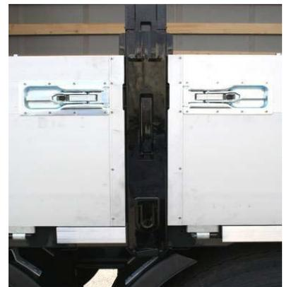
Side walls: Check that rivets are tight,
