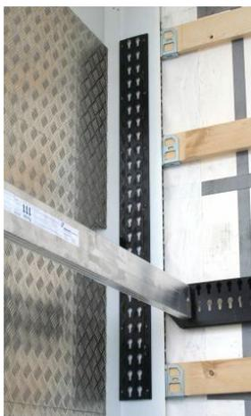
Front corner post: Check that the rail rivets are tight
