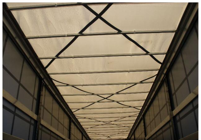
Strap reinforced roof tarpaulin: Check for damage and correct attachment
