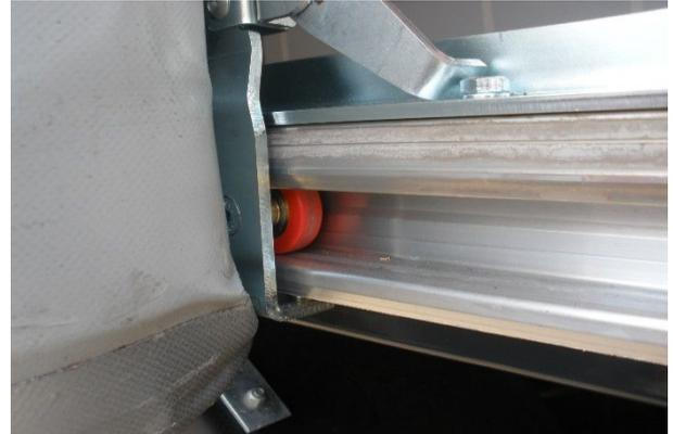
Visual inspection of Quick Slider for plastic deformation etc. Check bottom joints and carriages for wear and correct operability, check that screw fitting is tight
