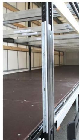
Central side posts, bottom: Check that rivets are tight
