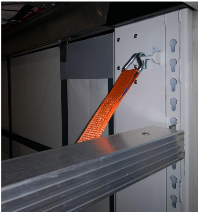
Hooking profiles: Check for deformation
