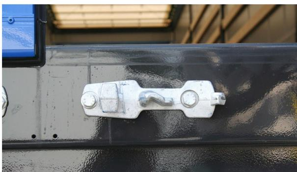
Bottom rear door: Check locking pin for damage and
