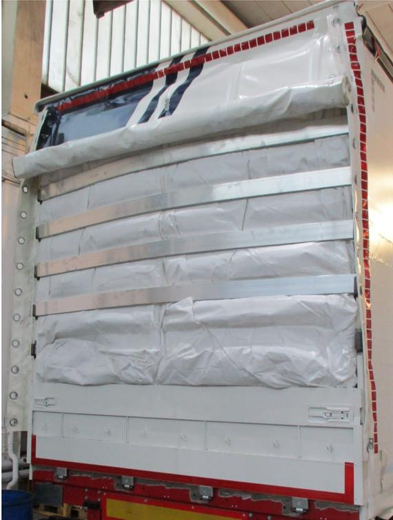
Check side panel, aluminium slats and their brackets for warping and damage.
