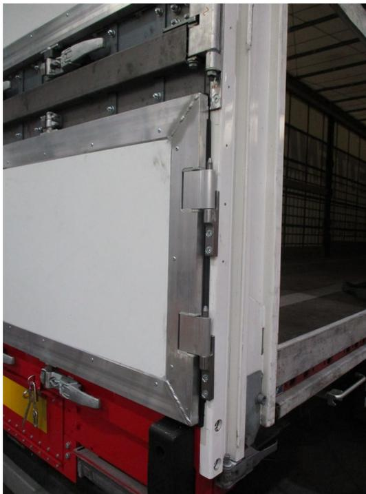
Check the hinges for operability and damage
