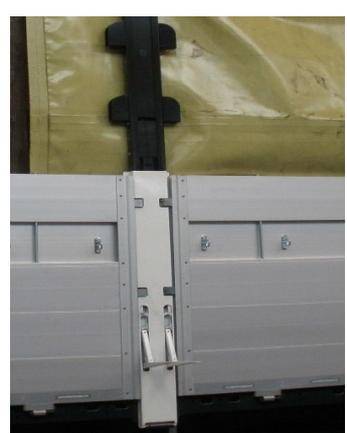
Side walls: Check that rivets are tight,
