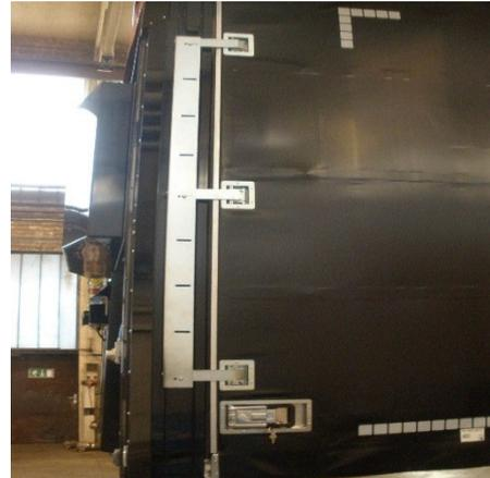
Quick Lock door: Check latch for wear and correct operability, mountability on rear corner post
