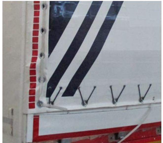
Check that strap feedthrough sleeves are not ripped,
