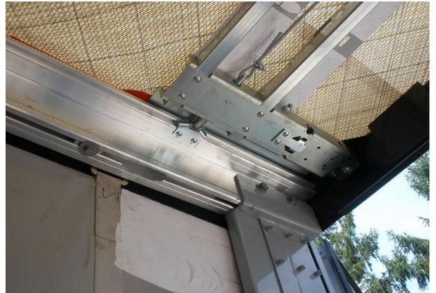
Aramid reinforced roof tarpaulin: Check for damage and correct attachment
