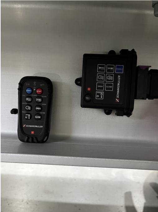
Radio remote control with control of work lights or lift axle
