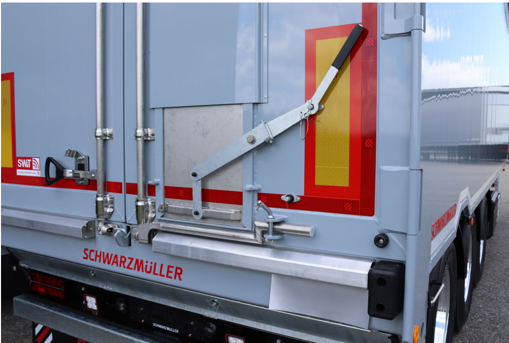
Tarpaulin protection board to protect the roll-up tarpaulin during the loading process
