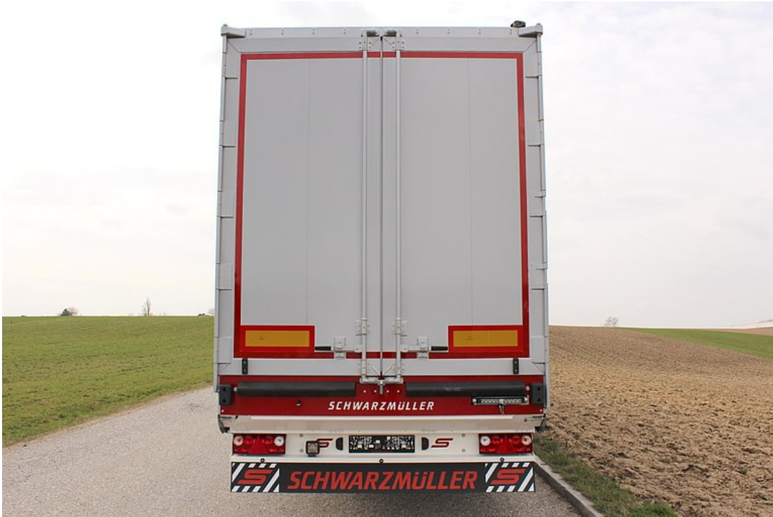
Rear wall = two-leaf door with one espagnolette on the outside of each door leaf and additional pneumatically operated safety lock
