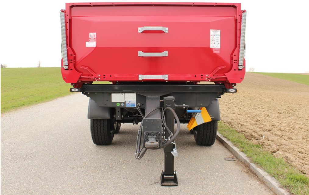
Steel sheet front wall with step on inside and outside
