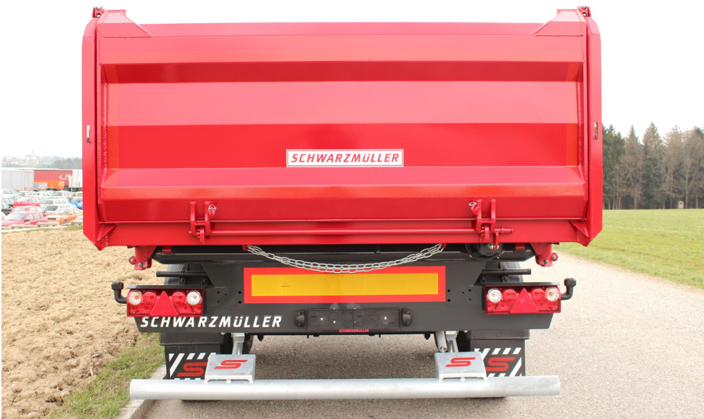
Steel sheet rear wall, hinged with raised bearing and autom. pneumatic lock
