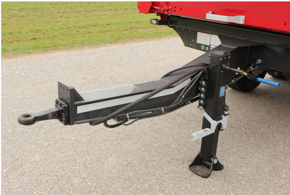
Foldable, tubular underride protection, with bumper block for road-finishing use
