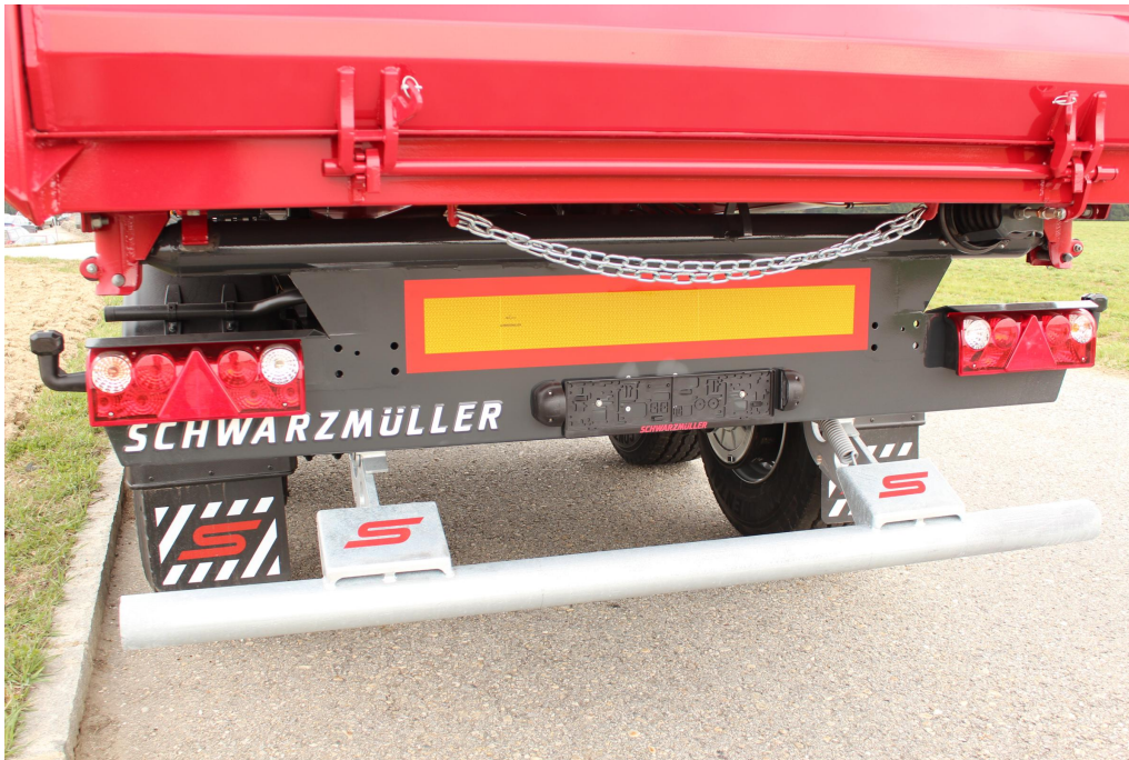
Foldable, tubular underride protection, with bumper block for road-finishing use
