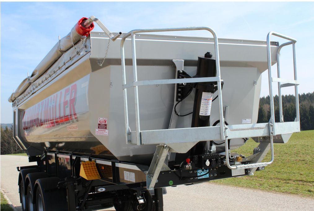
Optimum load distribution thanks to slanted front wall
