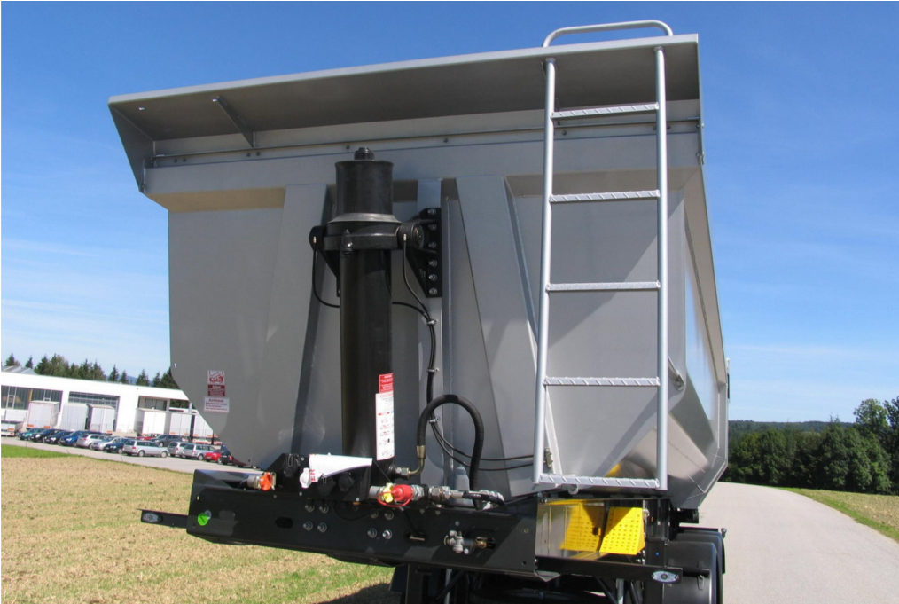
Optimum load distribution thanks to slanted front wall
