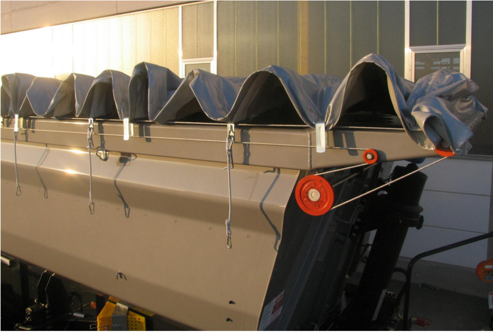
OPTIONAL: Roller cover - operated manually or via electric remote control
