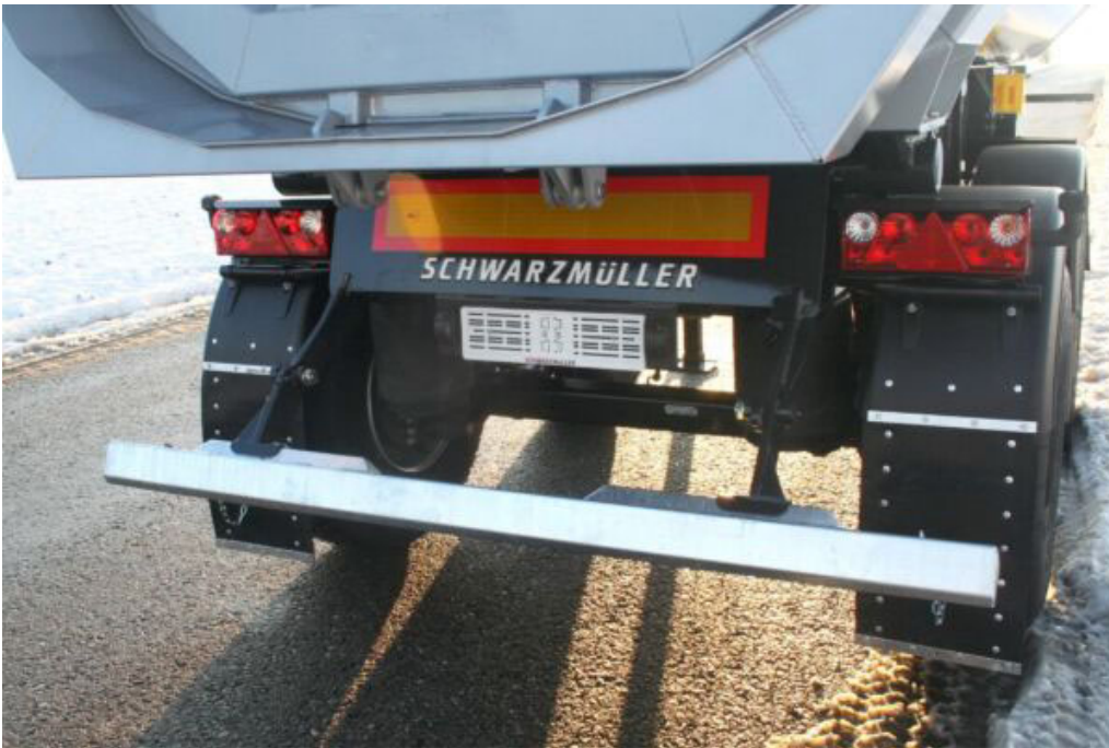
Foldable aluminium trapezoidal underride protection
