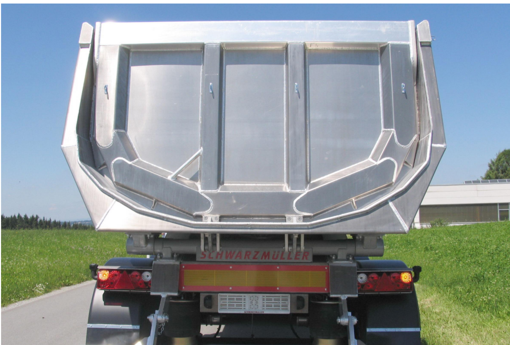
2-axle full aluminium segment tipper semitrailer - wheelbase 1,810 mm
