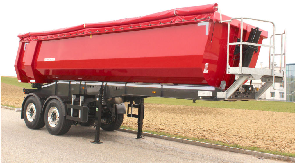
2-axle aluminium segment tipper semitrailer
