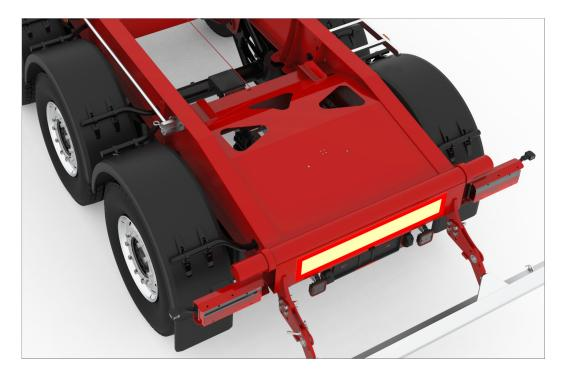
Torsion box: A proven and sophisticated solution ensuring perfect stability in the rear end area of tipper semitrailers
