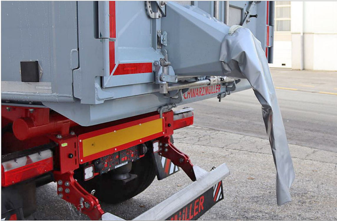
OPTIONAL: Dust bag: Simple means of avoiding the formation of dust.
