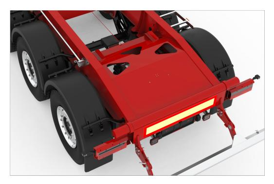
Torsion box: A proven and sophisticated solution ensuring perfect stability in the rear end area of tipper semitrailers throughout the entire tipping process.
