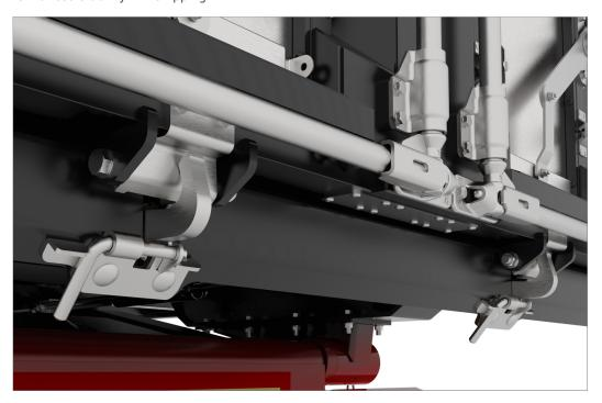
Automatic hinged door/flap latch: A special linkage assembly automatically unlatches the hinged rear wall then tipping and also re-latches it when lowering the box.
