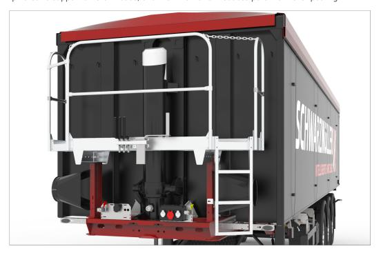
OPTIONAL: Platform: Use the platform to climb the box, monitor the loading process and open or close the tarpaulin.
