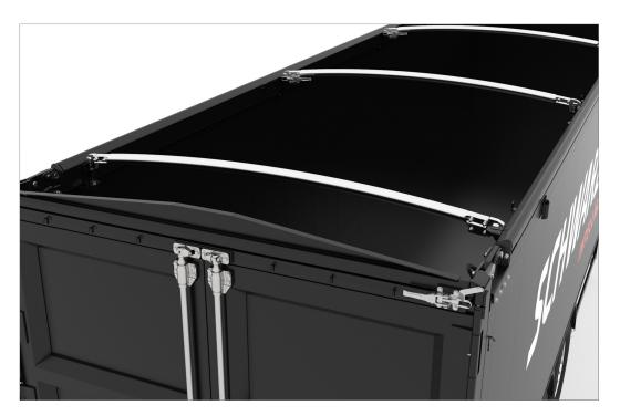
Cambered roof bar: The material-repellent roof bar are cambered to add stability to the tipper box. They can be pivoted to support different loads, and their inclination reduces potential water pooling.
