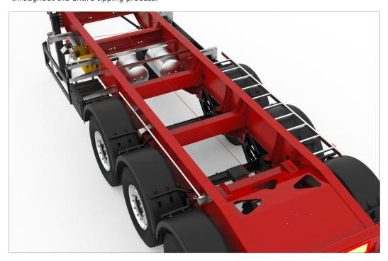
Torsion shafts: These special cross members work like the torsion box to add extra stability to the tipper semitrailer throughout the entire tipping process.
