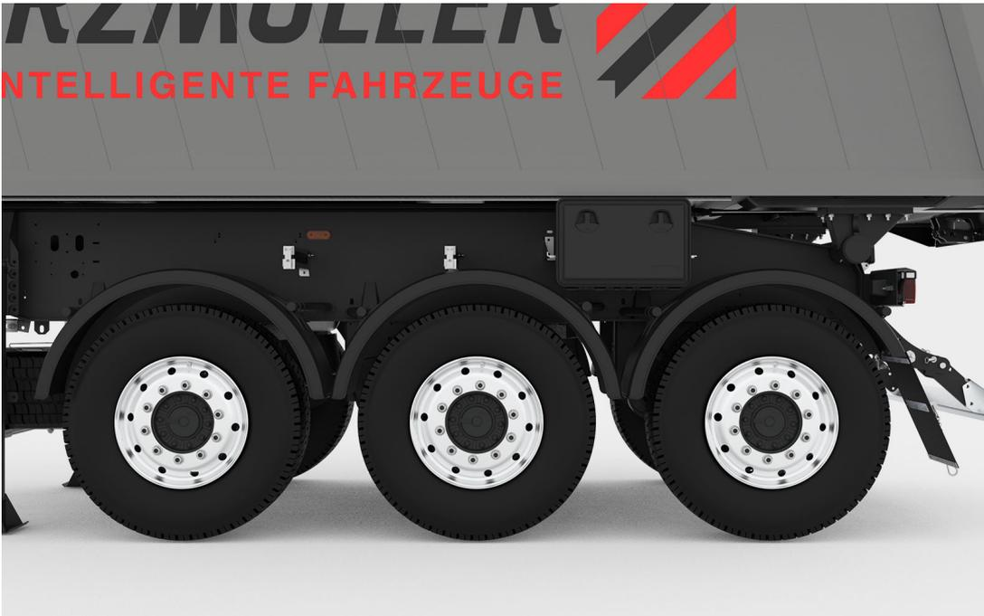
Schwarz Müller tipper semitrailers feature single wheel mudguards. They protect both other road users and the tipper box against road stone and dirt.
