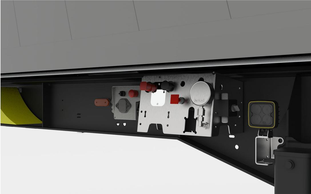
Arrangement shared by control elements such as brake release valves, lifting and lowering mechanism, trailer monitoring or lowering lock for easier use.
