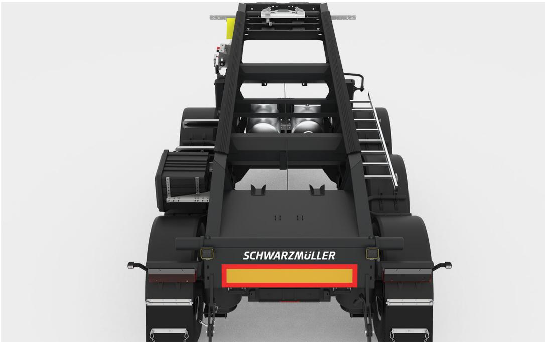
An advantage Schwarz Müller vehicles have over many competing products is the parallel arrangement of both longitudinal frames. as it provides more stability in every situation.
