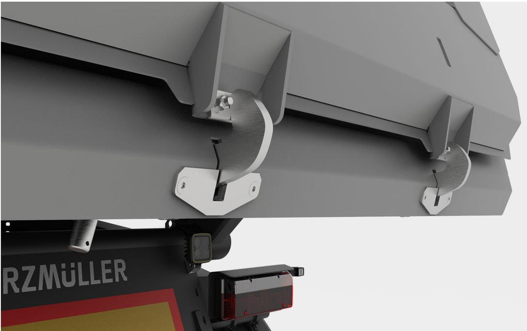
A special linkage assembly automatically unlatches the hinged rear wall then tipping and also re-latches it when lowering the box.
