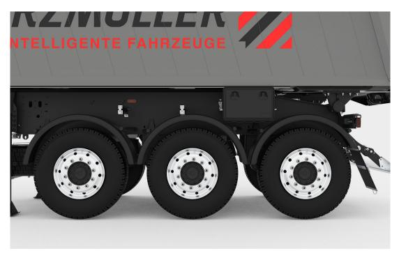
Schwarzmüller tipper semitrailers feature single wheel mudguards. They protect both other road users and the
