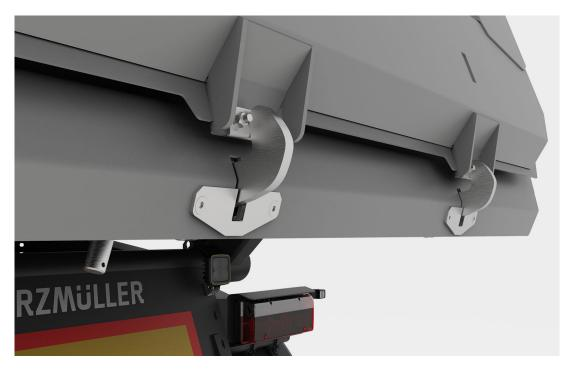
A special linkage assembly automatically unlatches the hinged rear wall then tipping and also re-latches it when
