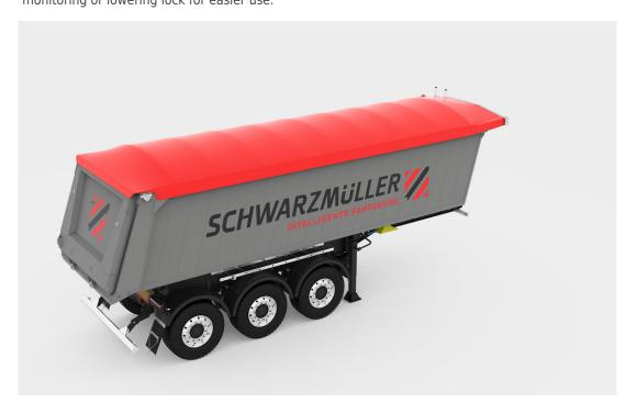
Electrically operated and remote-controlled sliding roof that conveniently opens and closes without having to climb
