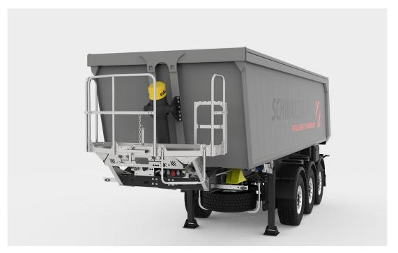
Use the platform to climb the box, monitor the loading process and open or close the tarpaulin.
