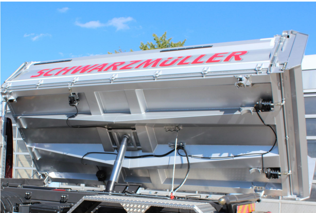
Stable and torsionally rigid chassis design with additional torsion tubes for 3-way tipping
