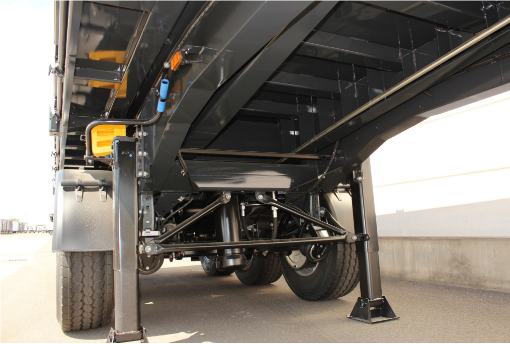
Stable and torsionally rigid chassis design with additional torsion tubes for 3-way tipping
