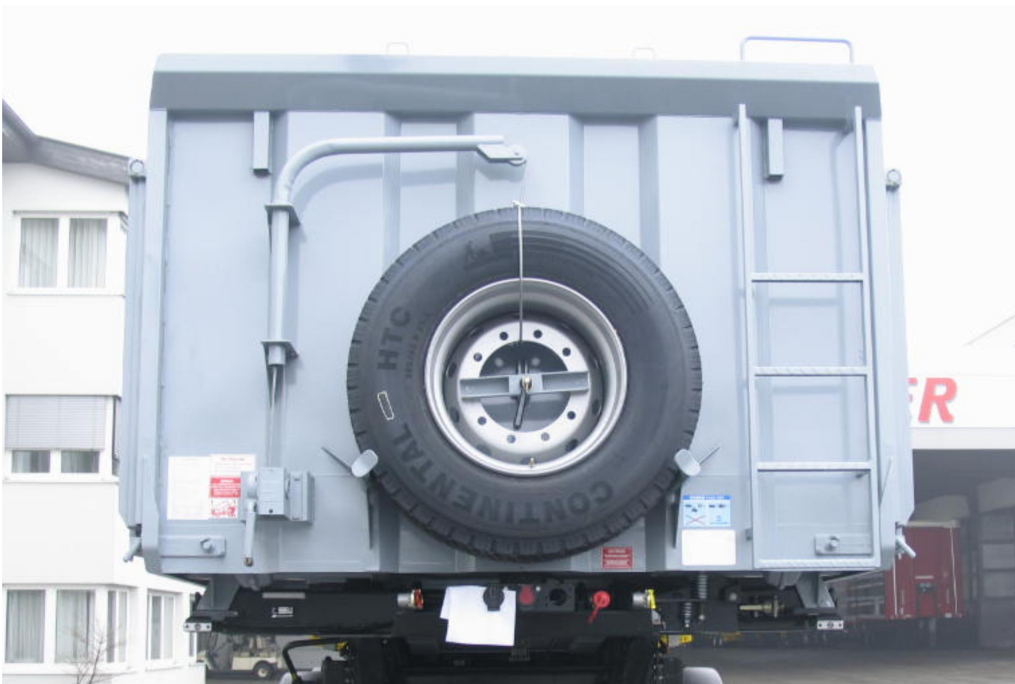
Manual central locking to open the side walls using a lever and central locking shaft
