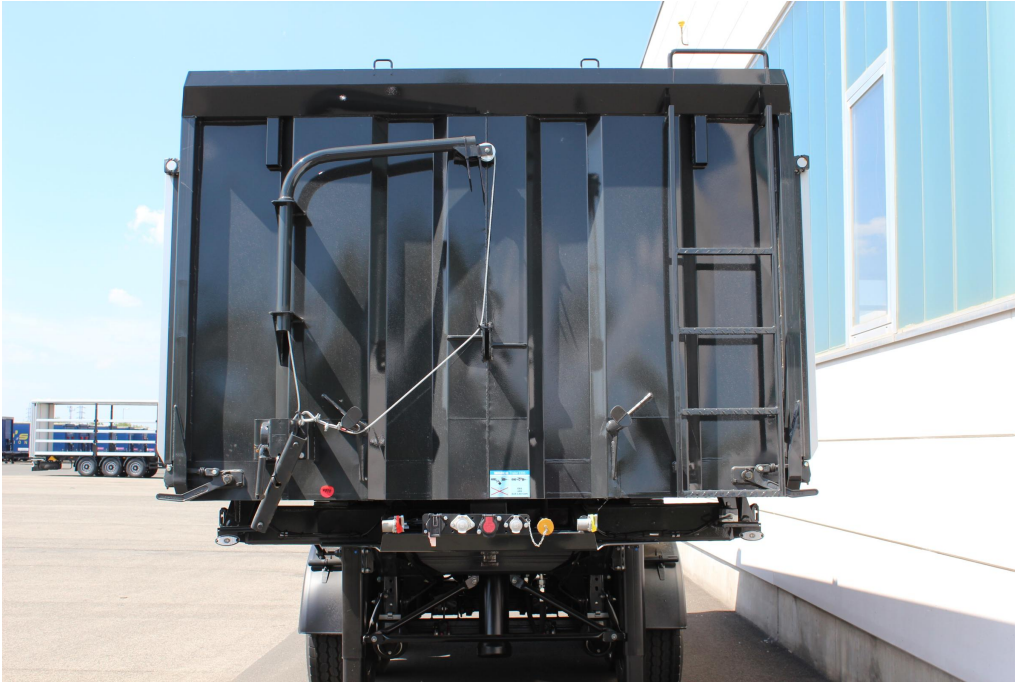
Fixed steel sheet front wall with lashing eyes, ladder and retaining brackets
