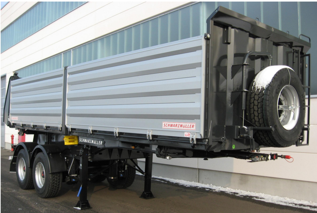
Fixed steel sheet front wall with lashing eyes, ladder and retaining brackets
