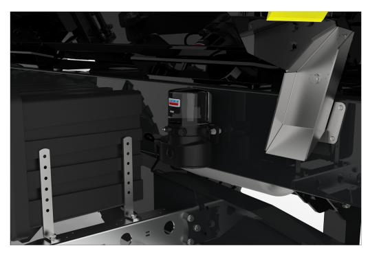
OPTIONAL: The central lubrication unit provides the entire vehicle with the required lubrication.
