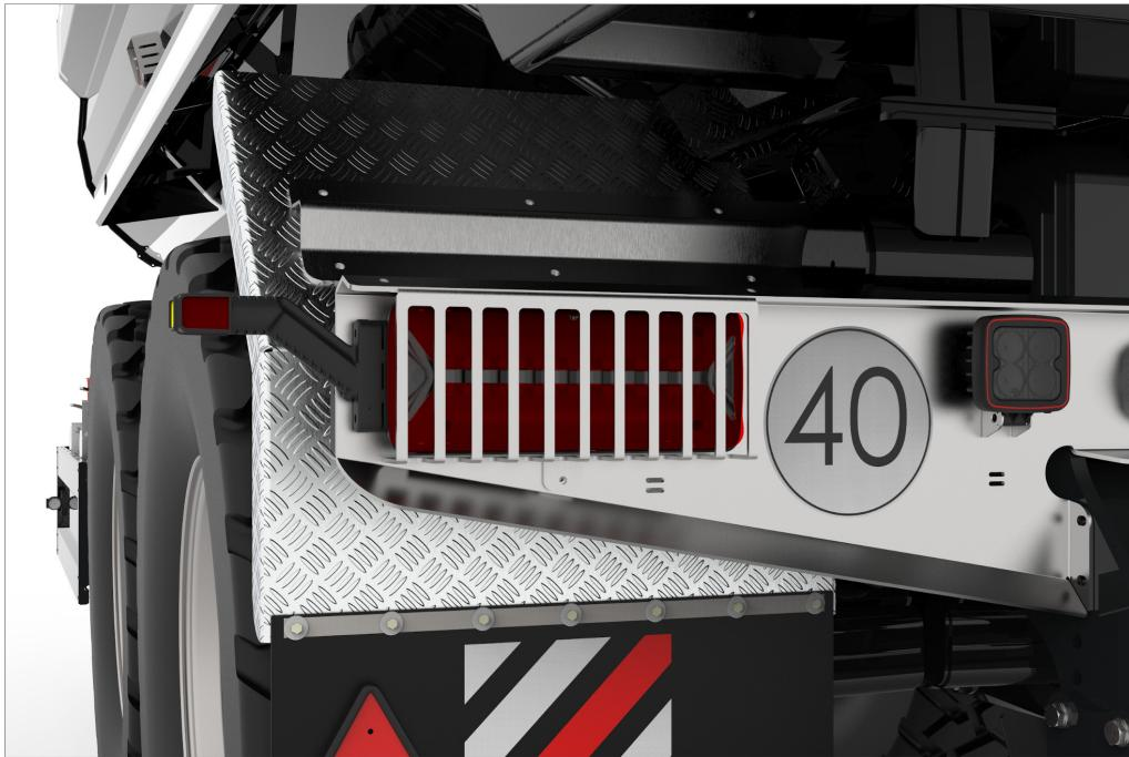
OPTIONAL: The LED tail lamps are mounted in a protected place. Their removable wire mesh guard enhances the safety of every service use (wire mesh guards not permitted on public roads).
