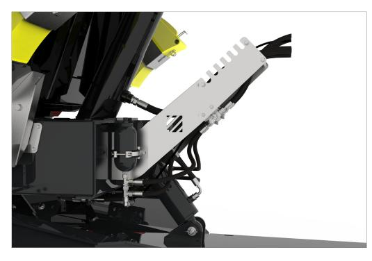
To ensure a perfect connection to the tractor, all connecting lines are protected in a hose duct.
