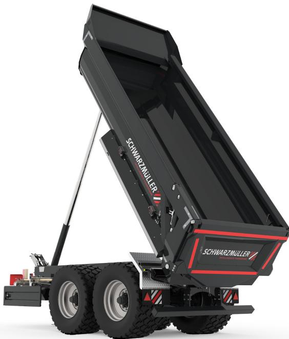
OPTIONAL: The heavy-duty rock tipper of abrasion-resistant steel (HB450) with 8 mm floor and 6 mm side walls will help you handle even the toughest jobs.
