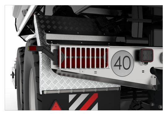
OPTIONAL: The LED tail lamps are mounted in a protected place. Their removable wire mesh guard enhances the
