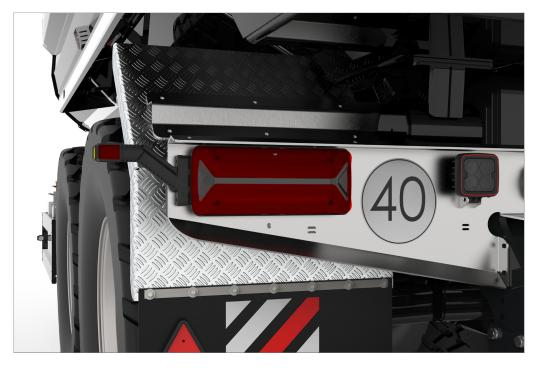
All light is produced by LEDs in vehicle lamps that are mounted in protected places and support multi-volt operation
