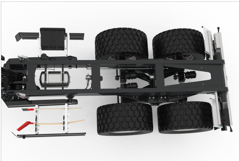
This special frame design of large profiled steel pipes is the main supporting element. Crossbars provide extra stability throughout the entire tipping process.
