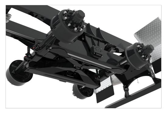
BPW's 30 t heavy-duty swing axle unit with bilateral axle load compensation plus its 650/55 R26.5" tyres ensure a
