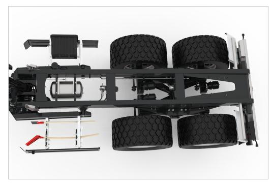
This special frame design of large profiled steel pipes is the main supporting element. Crossbars provide extra stability throughout the entire tipping process.
