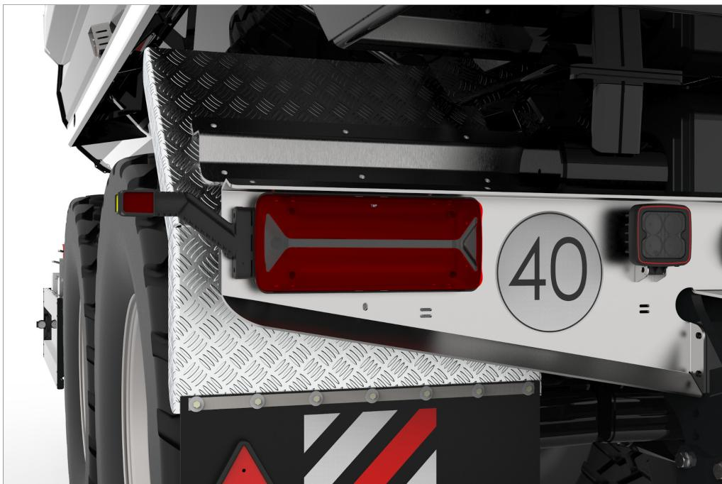
All light is produced by LEDs in vehicle lamps that are mounted in protected places and support multi-volt operation (12/24V).
