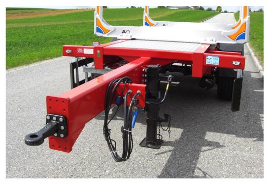
Height-adjustable drawbar for centre-axle heavy-duty coupling
