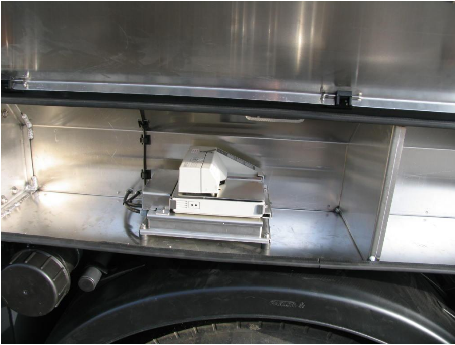
Aluminium box to protect the printer
