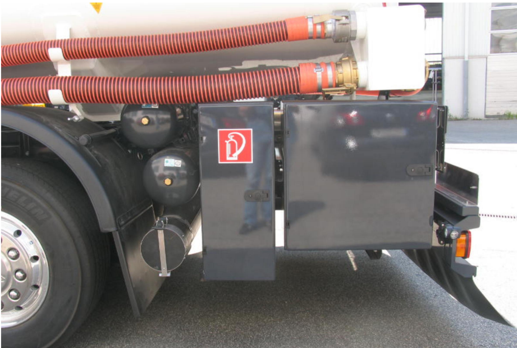
Aluminium box to protect the printer
