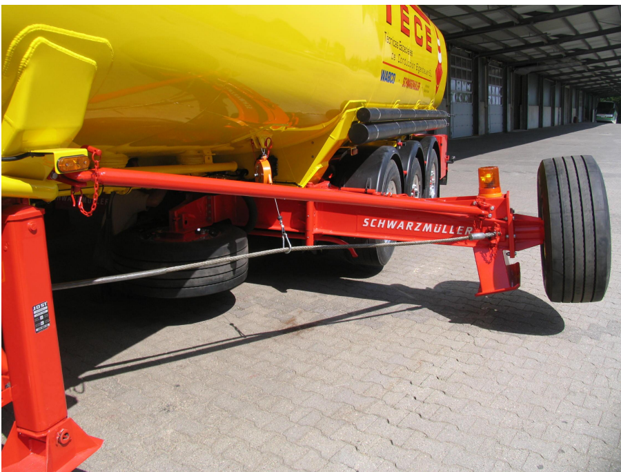
Arm with anti-kink device including anti-kink cables and revolving beacon on the right in the direction of travel
