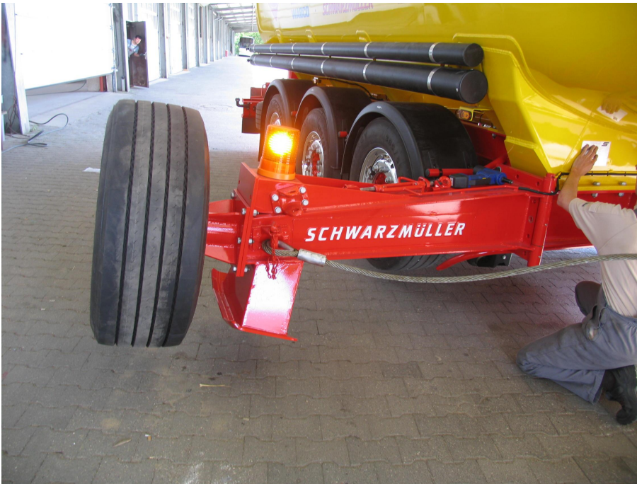
Arm with anti-kink device including anti-kink cables and revolving beacon on the right in the direction of travel
