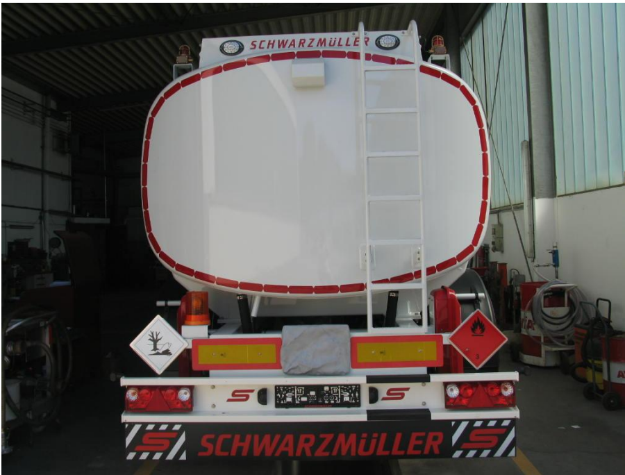
OPTIONAL: High-set lights integrated in dome tank
