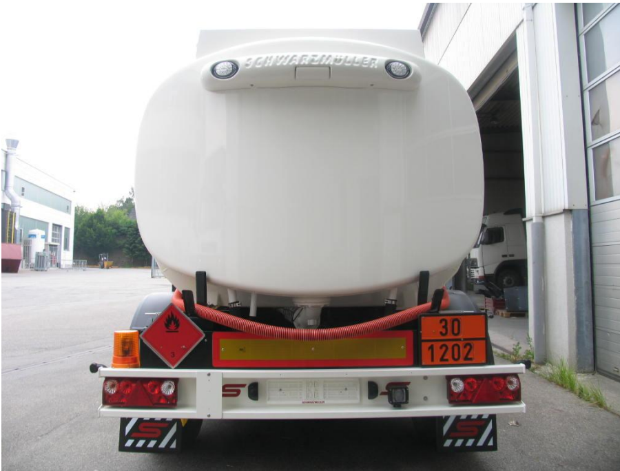
OPTIONAL: High-set LED light holder with optional integration of reversing camera
