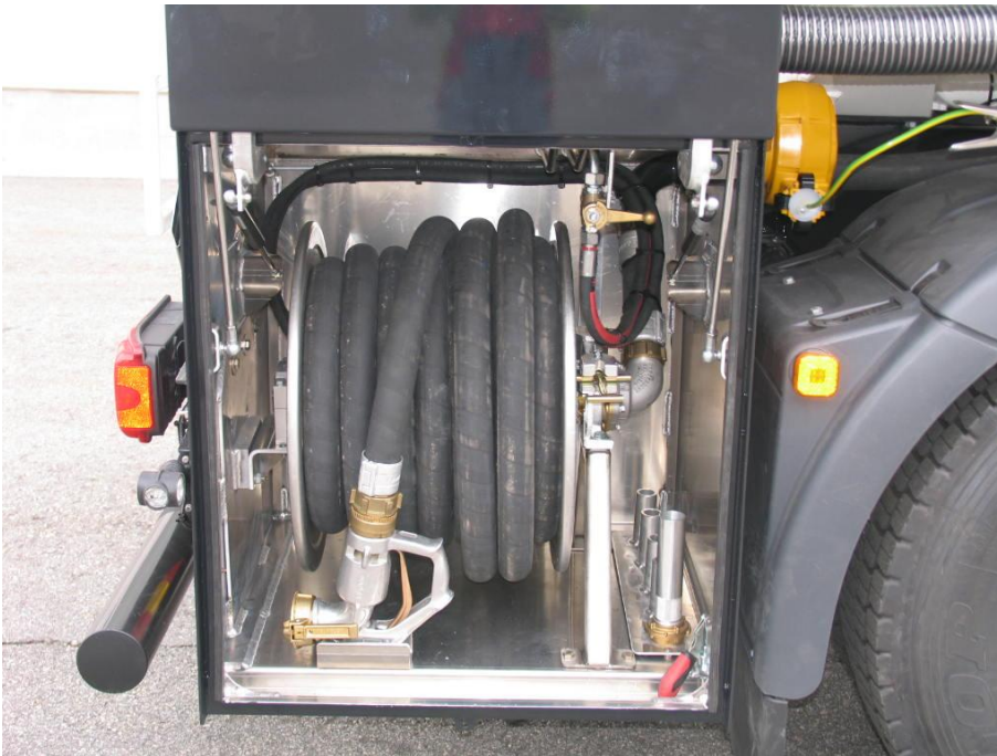
OPTIONAL: Ideal hose reel cabinet with parallel sliding door
