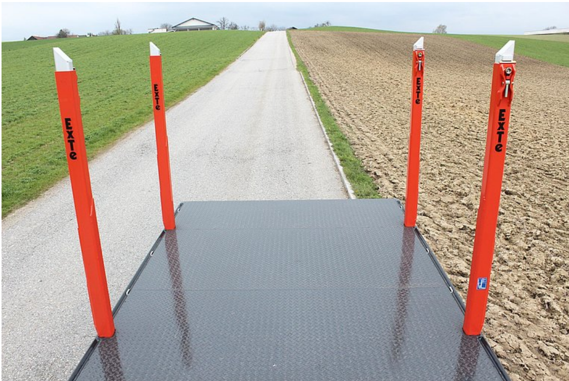
ExTe stanchion pockets with reinforcement brackets incl. 2-part ExTe stanchions 144-S with bolt fastening (load capacity: 7 t/pair)
