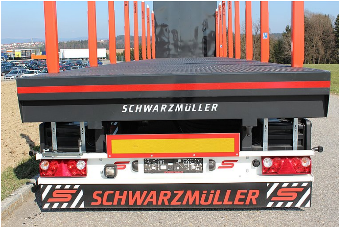
Rear closing element incl. fitted aluminium underide protection
