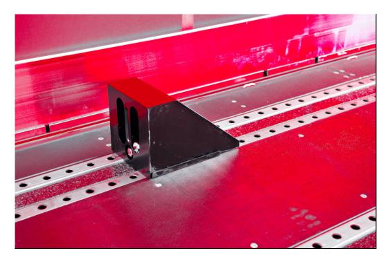
OPTIONAL: Load-securing wedges and Jolodarollers: Wedges with a spindle mechanism ensure that paper rolls are safely stored in transit. Use Joloda rollers for easily loading or unloading paper rolls.
