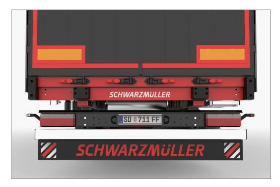
Underride protection: Prevents other vehicles from underriding the rear trailer end in conformity with new EU regulations coming into force in 2021 (higher test loads).
