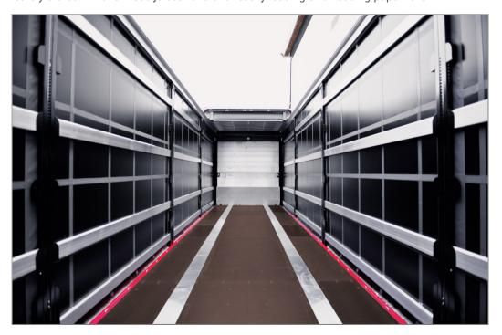
Force-controlled resin-coated floor: 28 mm + 12 mm (stacker axle load: up to 8,000 kg).
