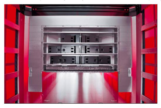
OPTIONAL: Wedge box (paper): The wedges for securing paper rolls in transit are kept in a box in the front wall.
