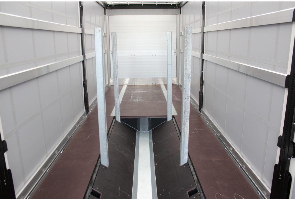
Manually operated hydraulic lifting roof, 400 mm elevation for rapid loading and unloading
