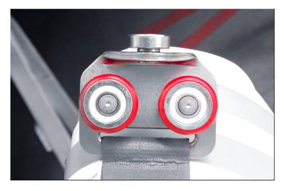
Trike Roller: For suspending the side tarpaulin. One horizontal and two vertical guide rollers make handling the
