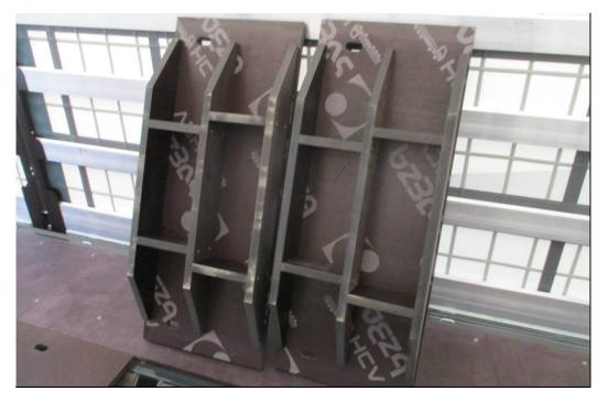
OPTIONAL: Coil trough cover panels: Used to cover the coil trough in general cargo use.
