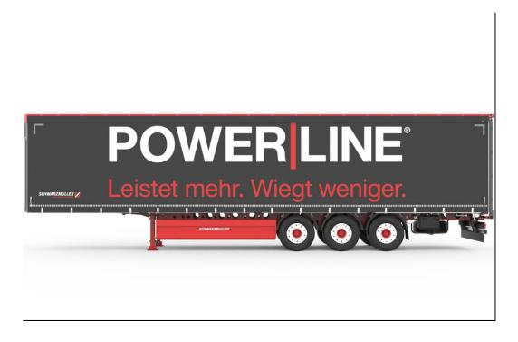
Low corrosion, high-quality aluminium body components, tested according to EN 12642 Code XL.
