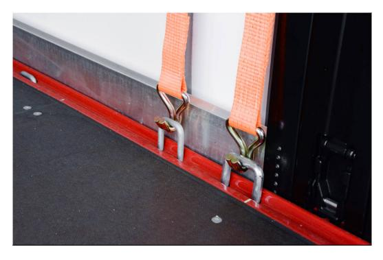
OPTIONAL: Lashing points on coil trough: Apart from the standard 2.5 t lashing points, there are also some extra 4 t
