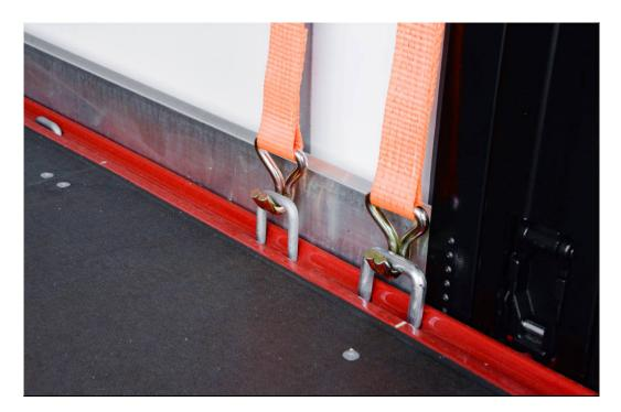
OPTIONAL: Lashing points on coil trough: Apart from the standard 2.5 t lashing points, there are also some extra 4 t points for securing the coil.
