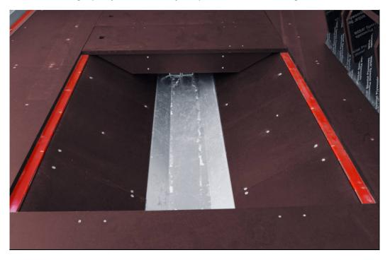
OPTIONAL: Coil trough: This trough set into the floor safely holds the steel coils in transit.
