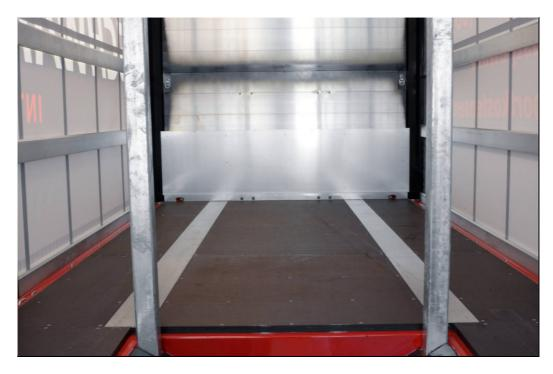
OPTIONAL: Upright frames of profiled steeltube for coil trough: These frames secure the coil in forward direction.
