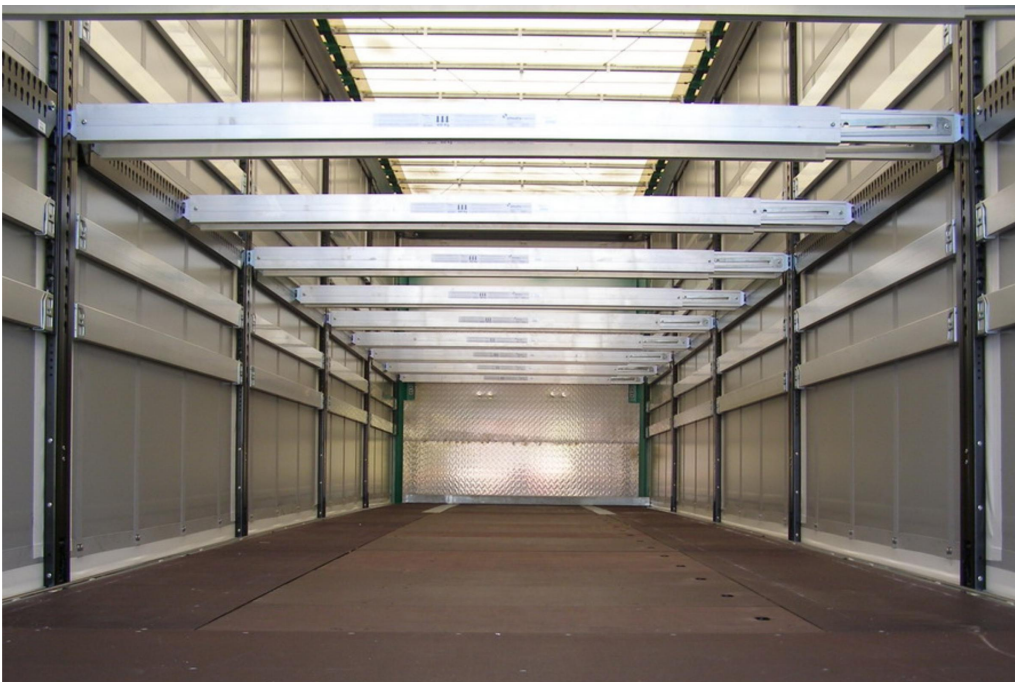
3-axle sliding tarpaulin platform semitrailer with twin-level loading system
