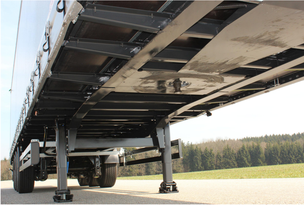
Torsionally rigid, welded ladder frame structure
