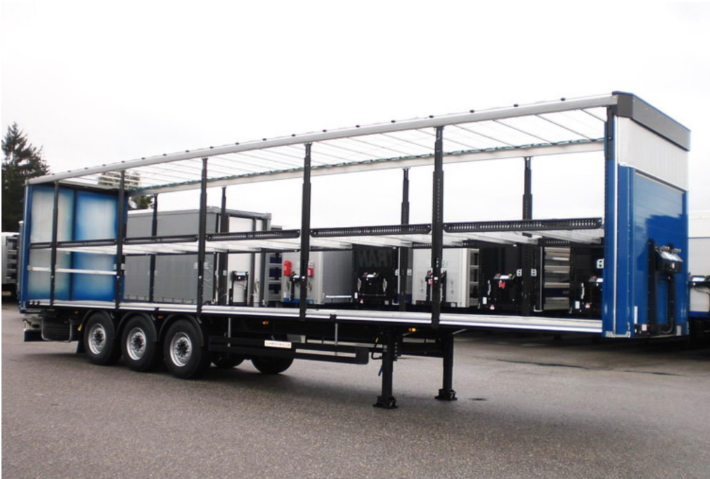
3-axle sliding tarpaulin platform semitrailer with twin-level loading system
