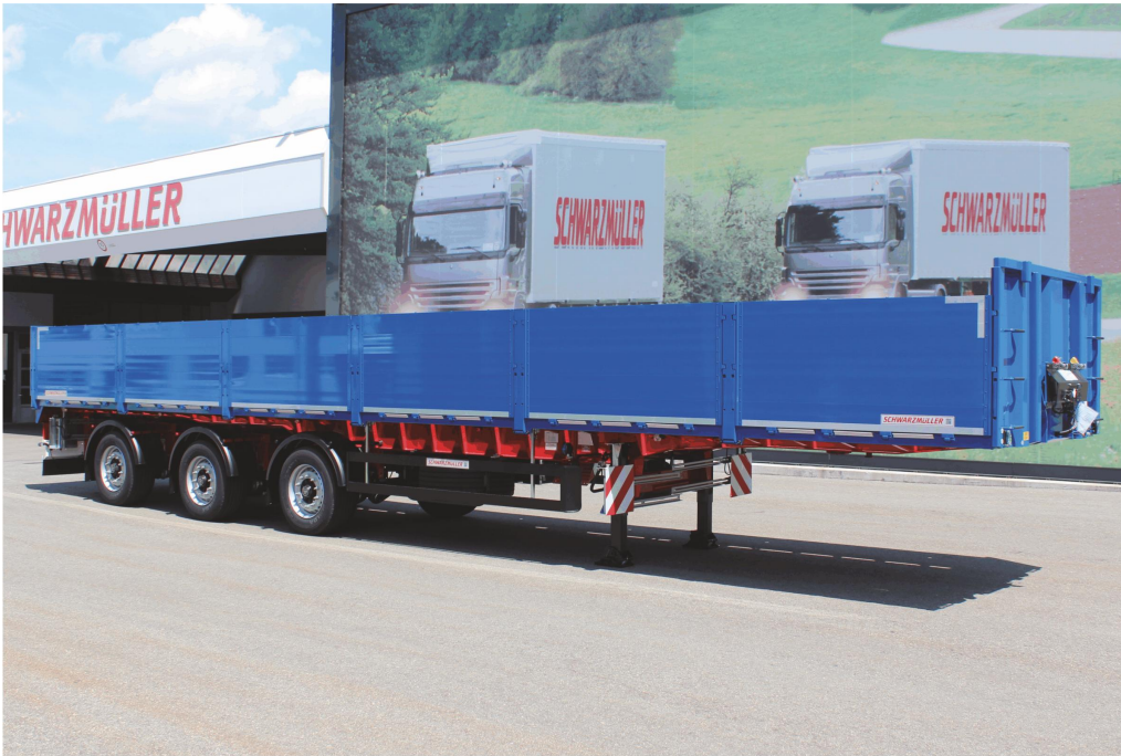
3-axle platform semitrailer with/for mobile crane
