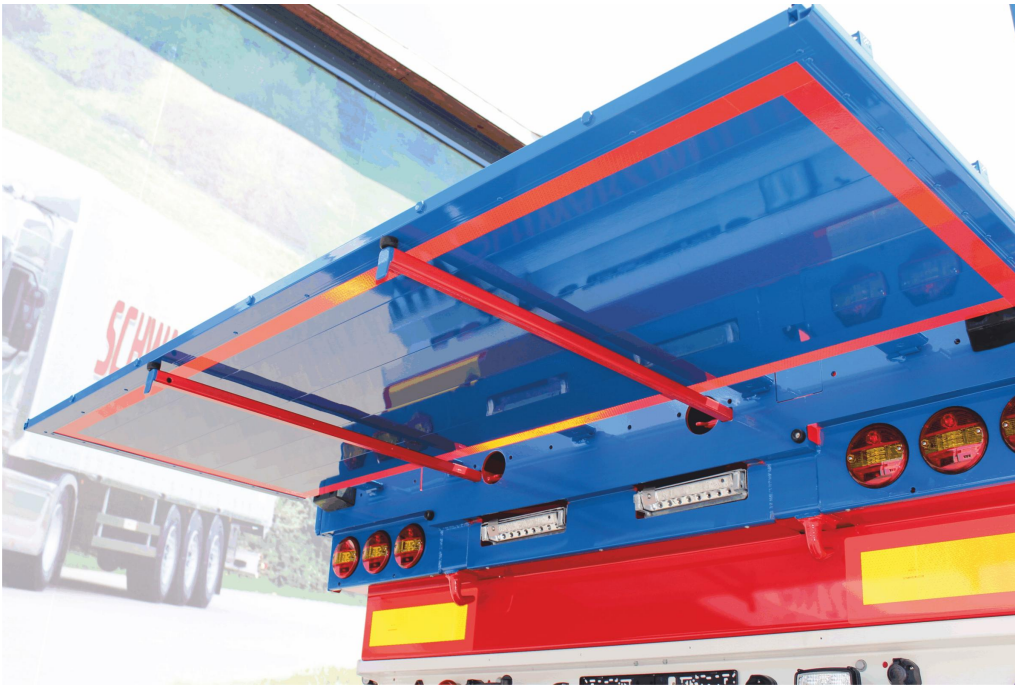
2 slide-out supports for rear wall (non-load-bearing)
