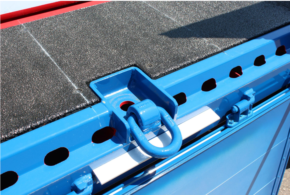
Perforated external frame with approx. 100 mm hole spacing, 50/30 mm slot, for securing 2 t
