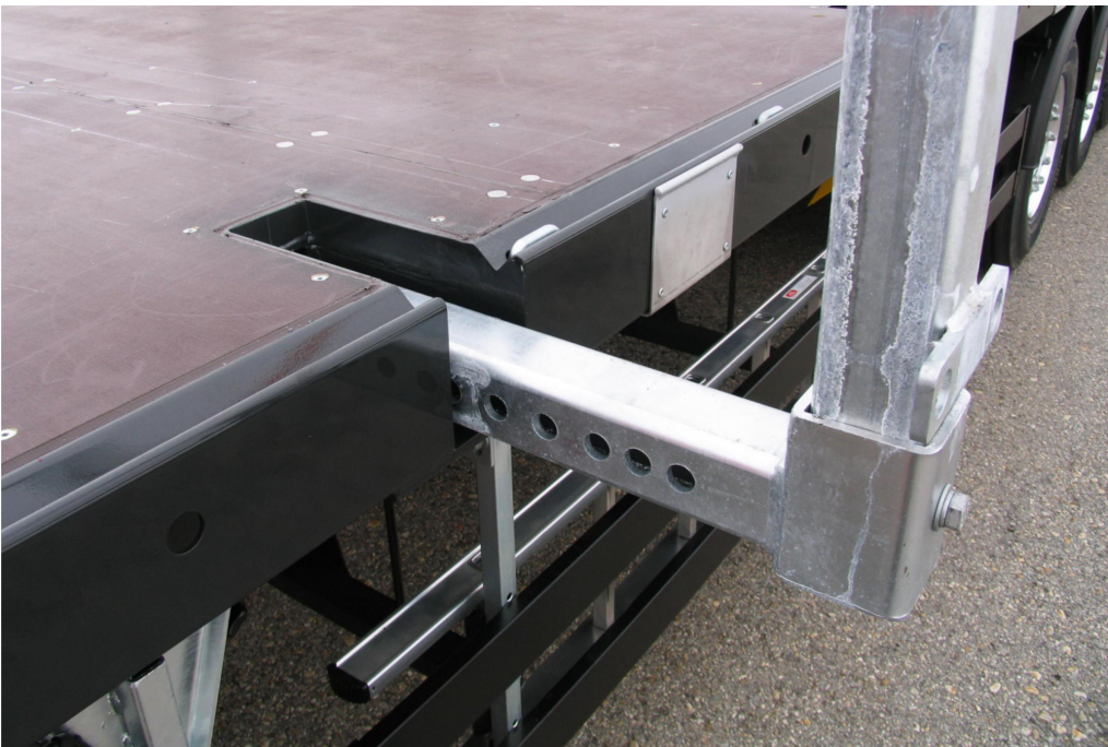
Rack positions for securing stacked construction steel mats, each with a length of 6,000 mm
