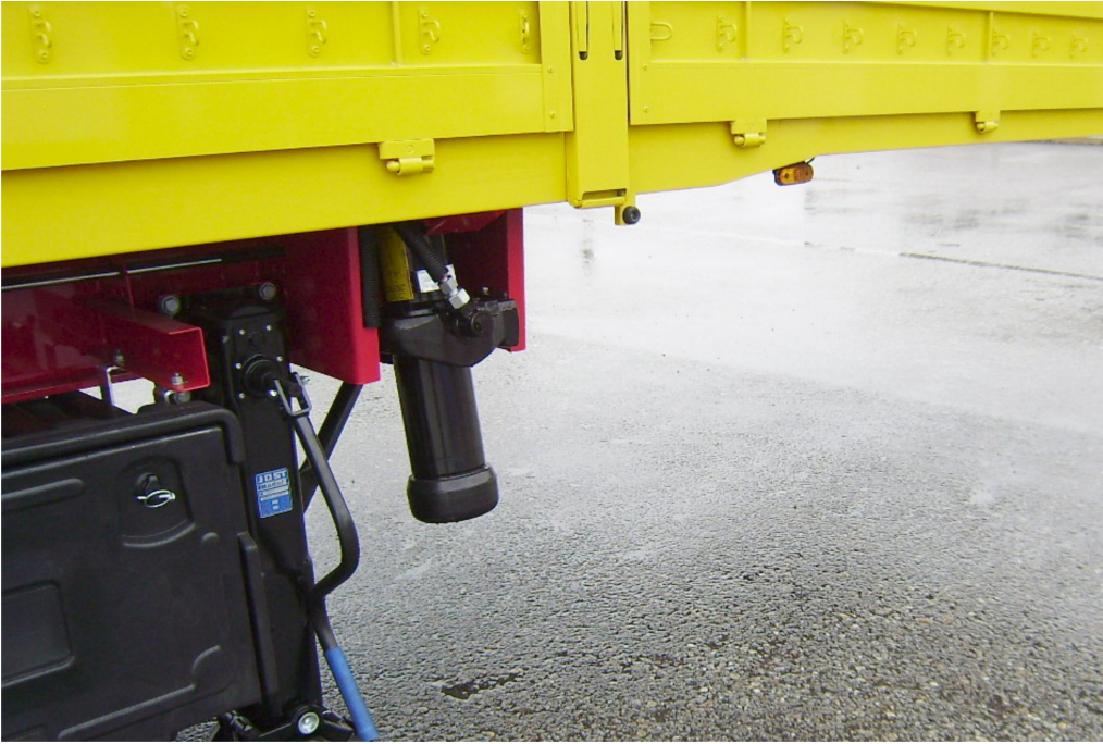
Electrohydraulic pump unit for independent operation of the inclined loading device on the semitrailer
