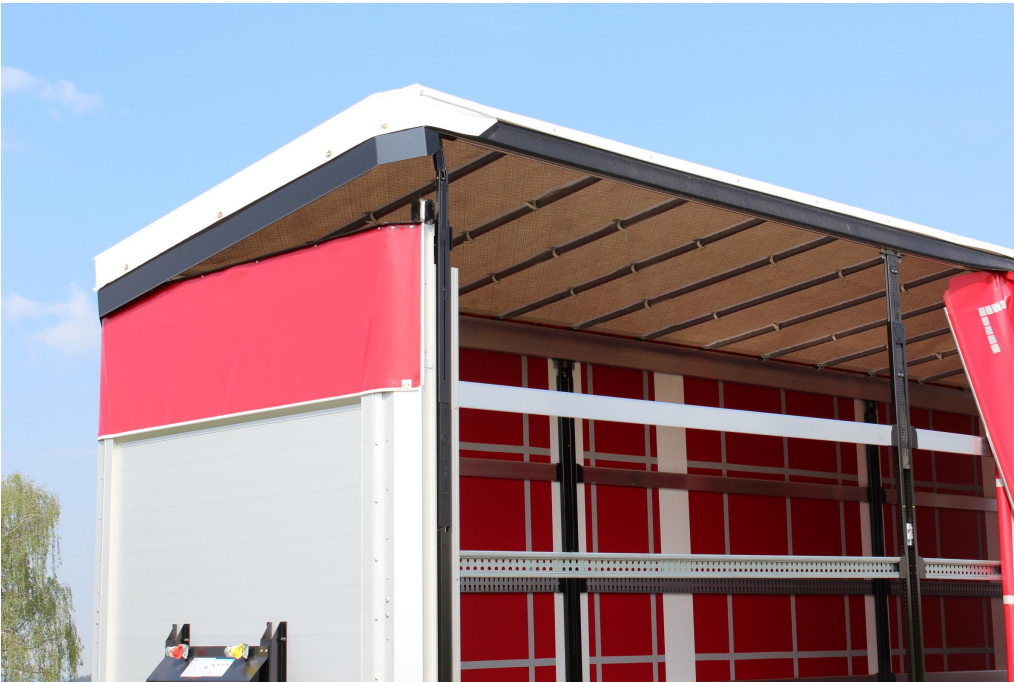
OPTIONAL: Twin-level loading system CTD III for 11 x 3 EURO pallets, load capacity: 400 kg/pallet
