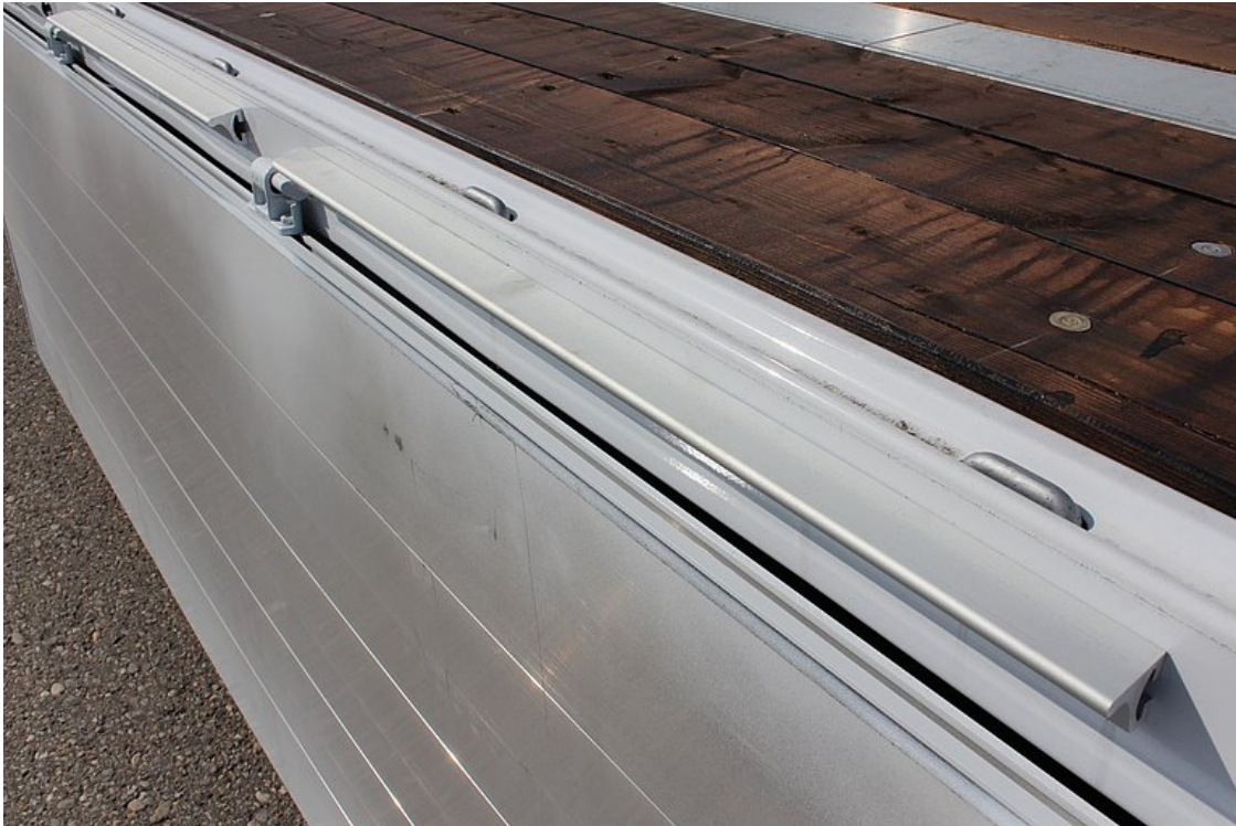
External frame with 15 pairs of recessed lashing points for load securing
