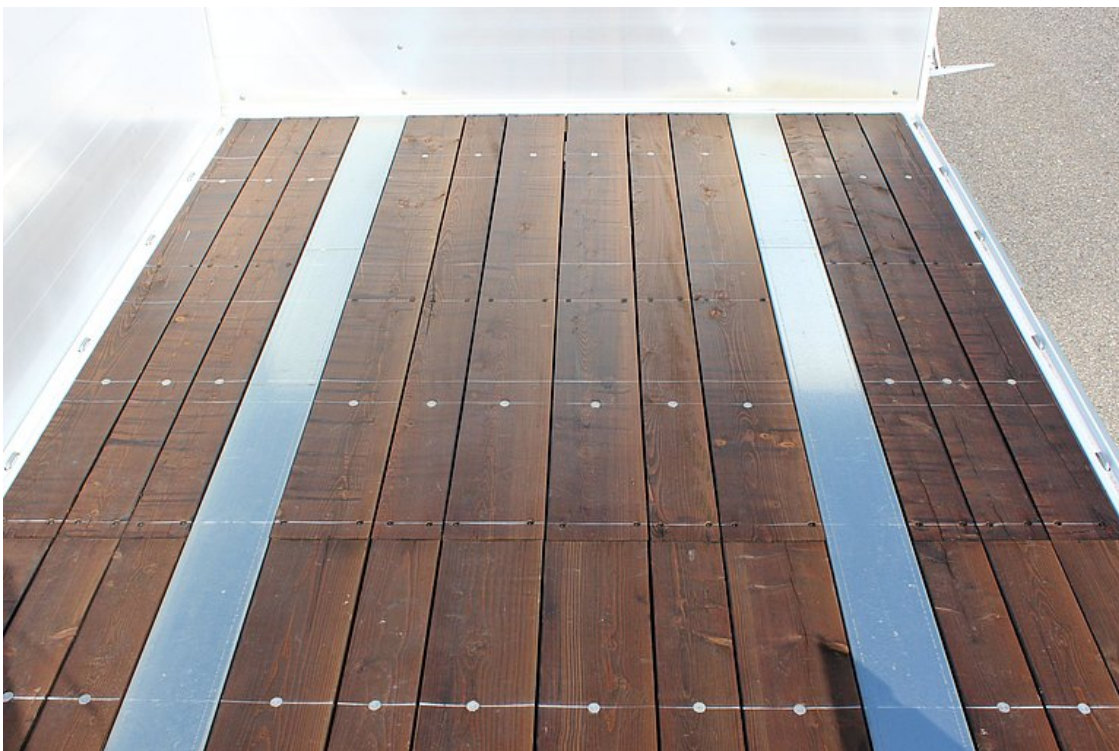
OPTIONAL: Weather-resistant larch wood floor 40 mm, without secondary floor
