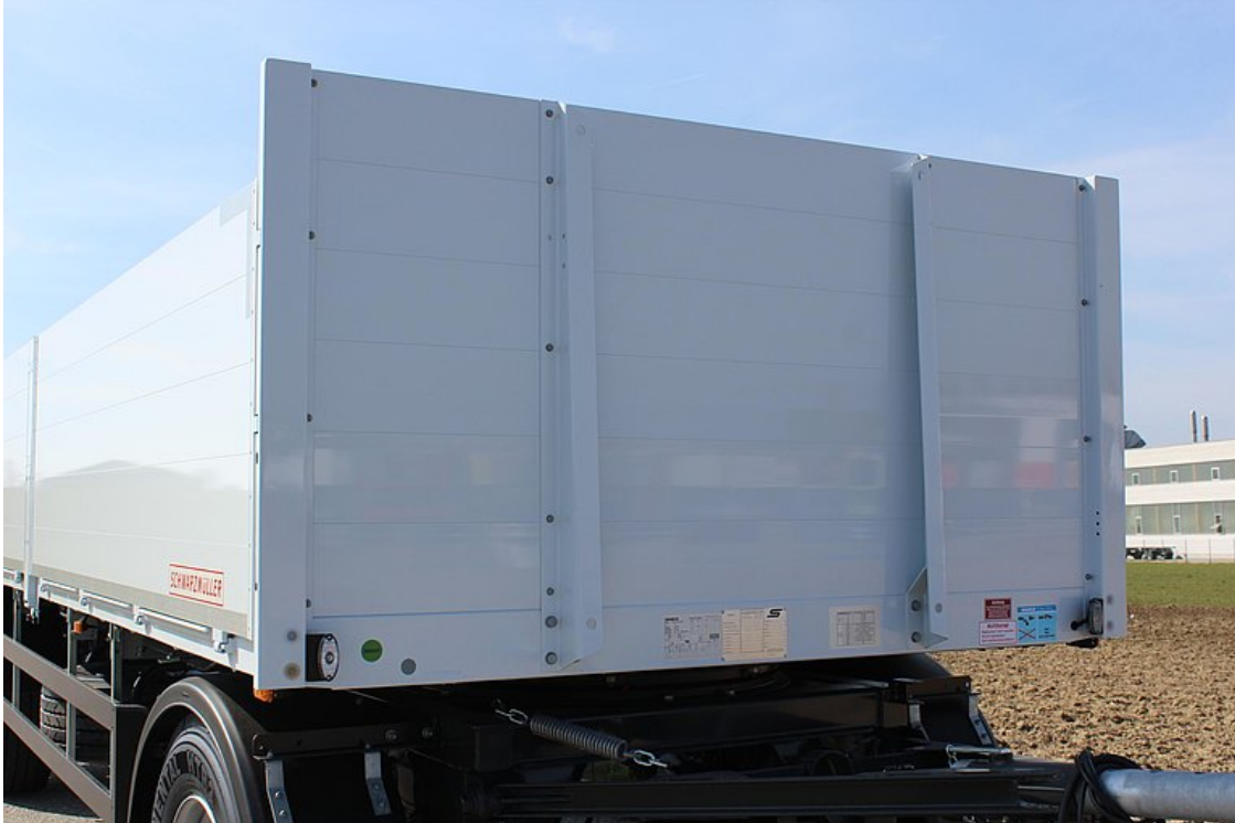
Fixed aluminium hollow profile front wall with 2 centre supports to the top
