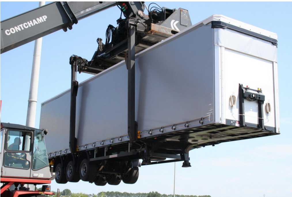
Reinforced frame construction with 4 grip edges for crane-based rail loading
