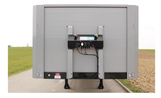
Fixed aluminium hollow profile front wall with 2 centre supports, inside with 2 lashing eyes for load securing and
