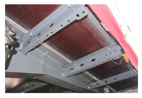
27-mm resin-coated panel floor, flush with external frame and with 2 steel top-hat profile rails above the side
