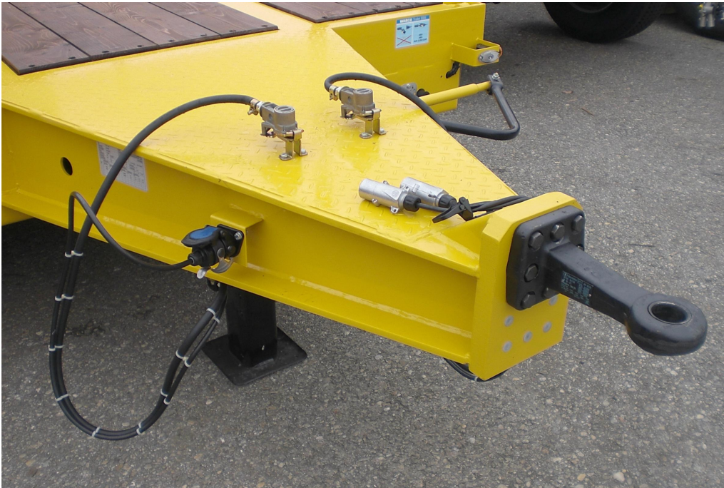
Drawgear contracted before bridge platform, with bolted drawbar eye
