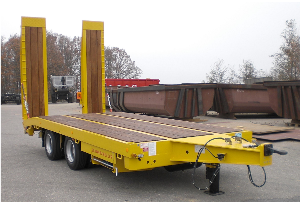
Drawgear contracted before bridge platform, with bolted drawbar eye
