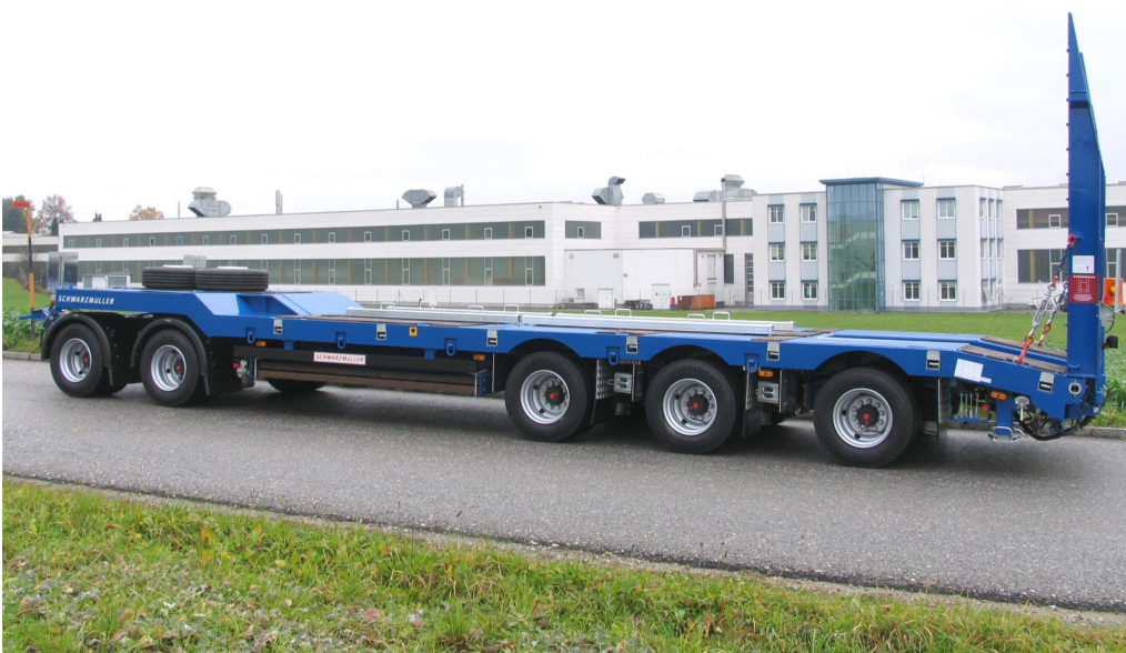
5-axle low loader trailer with offset platform
