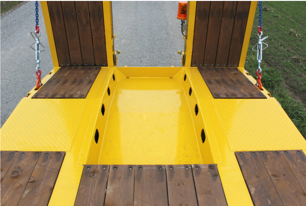
Pull-out extensions, on both sides of drop deck and rear taper, incl. extension planks for transporting wide loads
