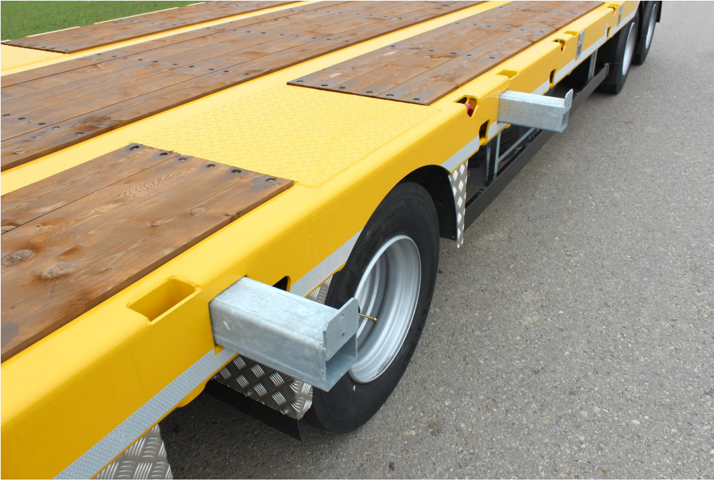
Pull-out extensions, on both sides of drop deck and rear taper, incl. extension planks for transporting wide loads
