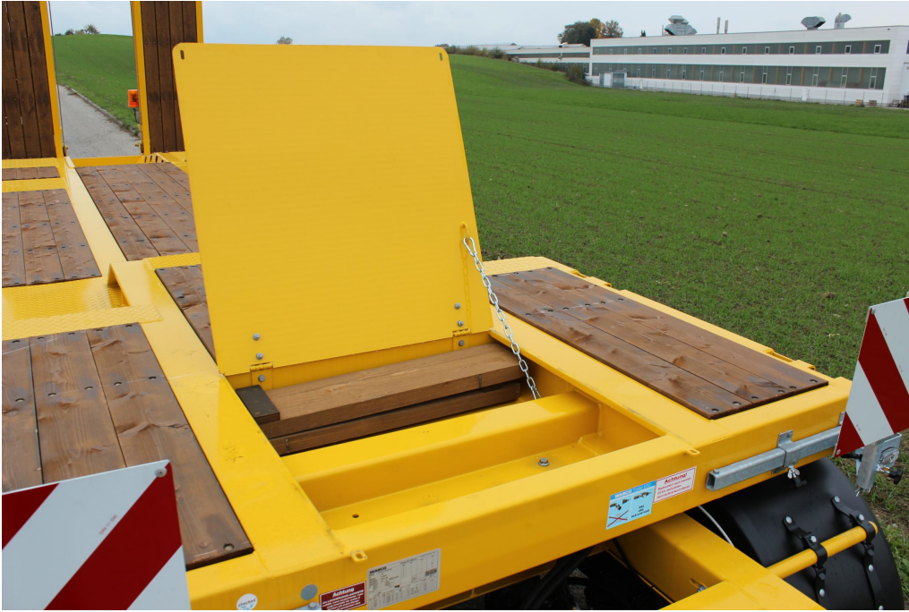
1 accessory compartment at front centre of raised platform, with folding lid
