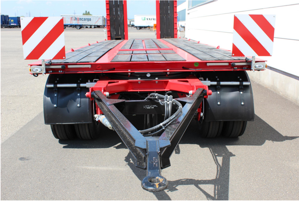
Bogie at front incl. drawbar and pull-out warning signs on frame for transporting wide loads
