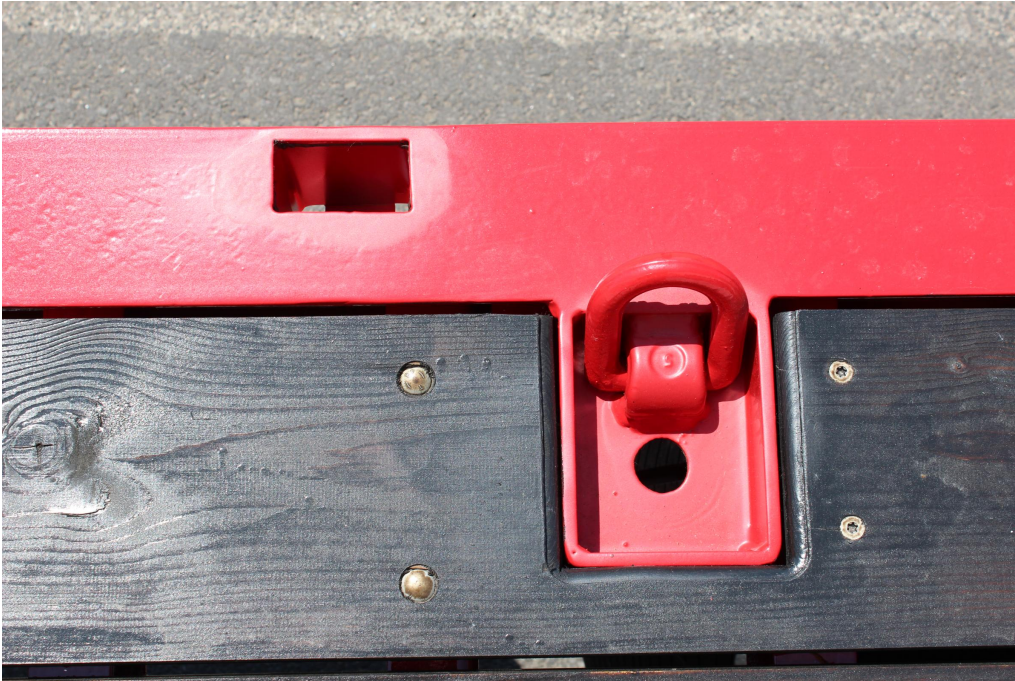
5 pairs of recessed, foldable lashing eyes
