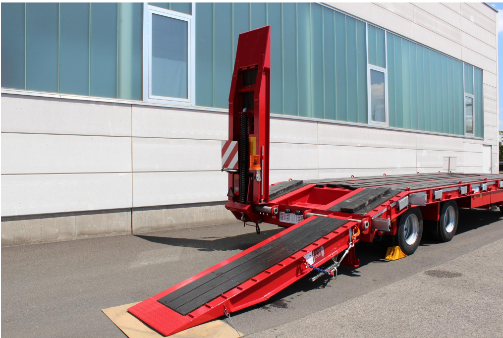
Bogie at front incl. drawbar and pull-out warning signs on frame for transporting wide loads
