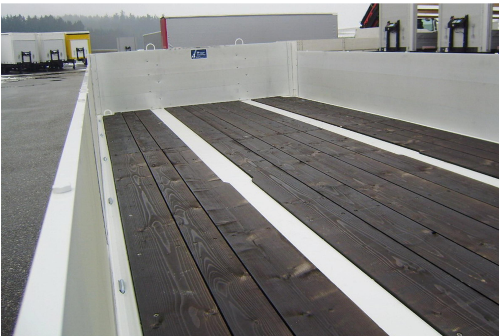
3-axle low loader trailer with straight platform
