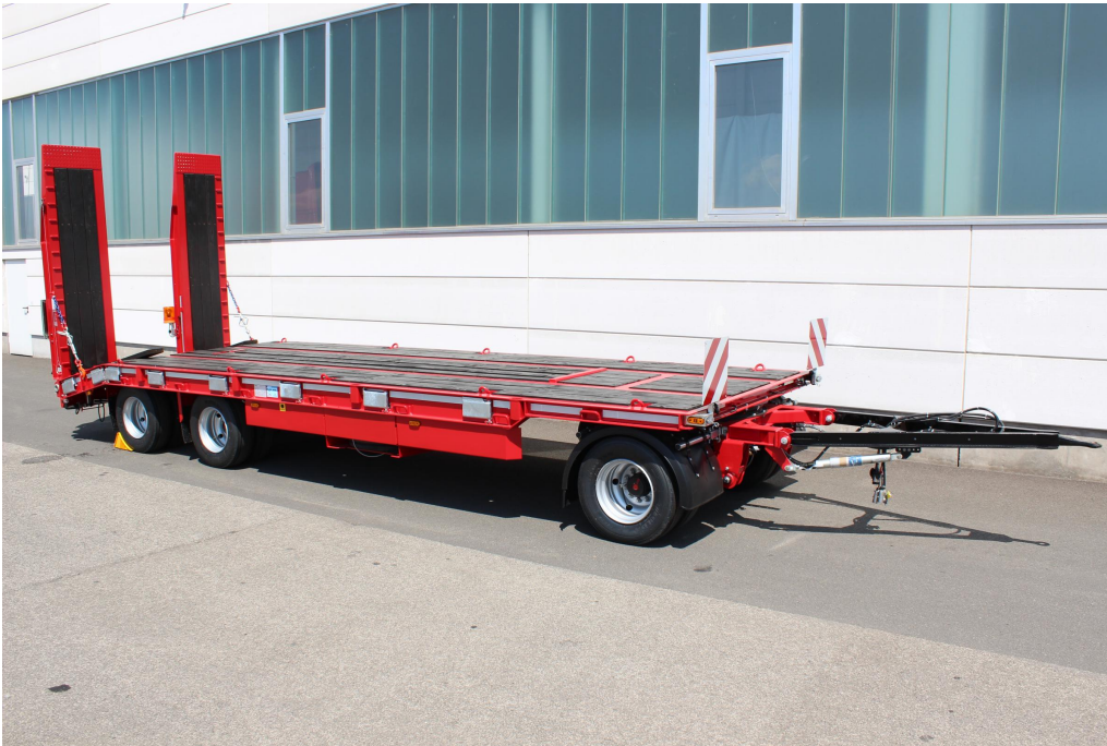
3-axle low loader trailer with straight platform
