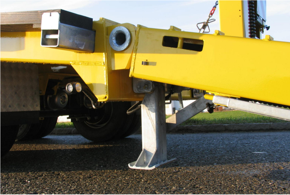
1 automatic folding support per ramp and frame end at rear end
