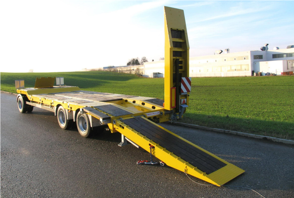
2 folding single-part loading ramps with hardwood flooring
