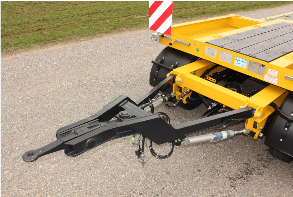
Offset drawbar with pivoting eye, 40 + 50 mm
