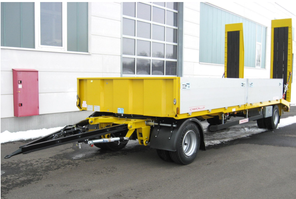
2-axle low loader trailer with straight platform
