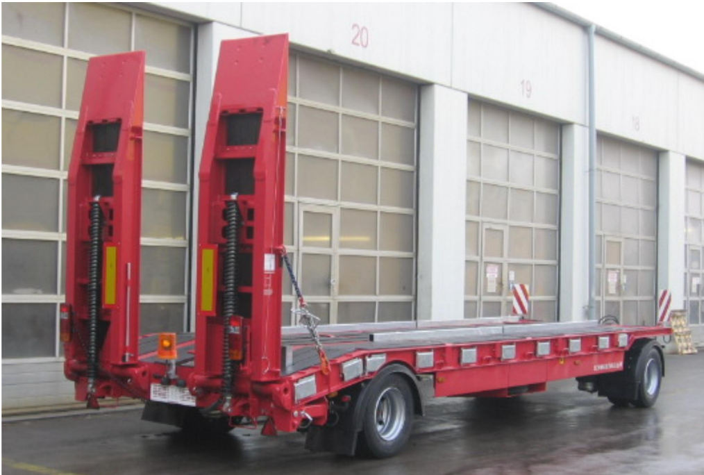
2-axle low loader trailer with straight platform
