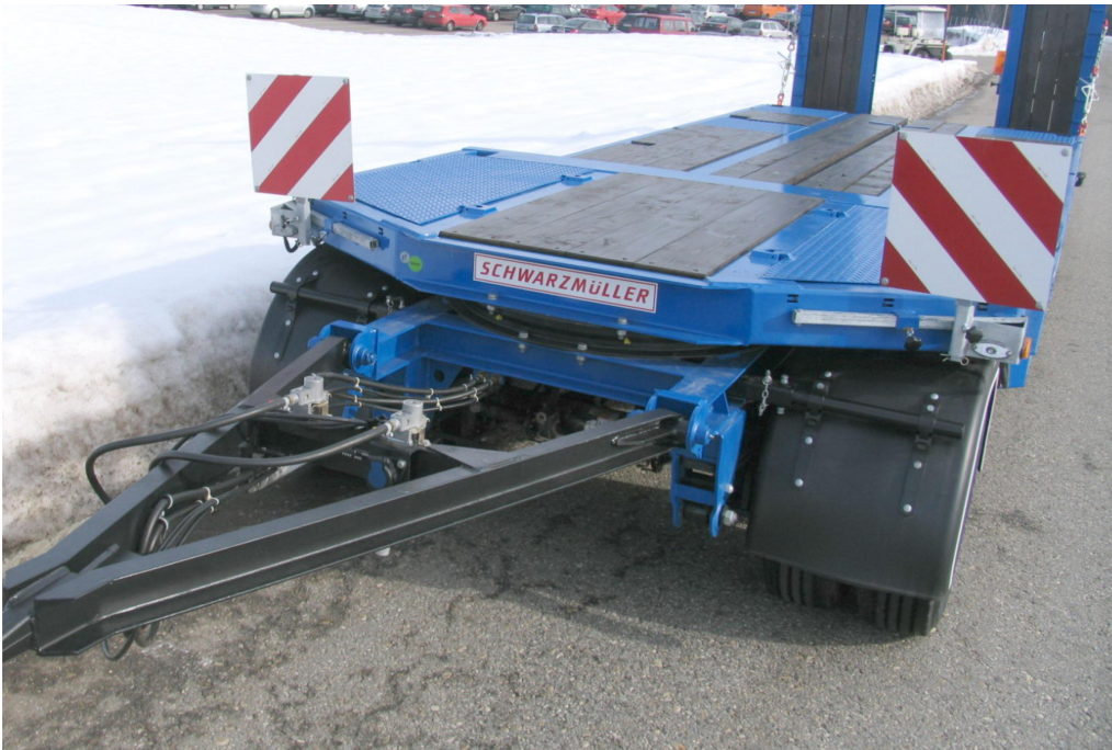
Bogie at front incl. drawbar - OPTIONAL: Pull-out warning signs for transporting wide loads
